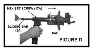
4. Squeezing the Trigger (6A) will force Sliding Bar (2A) forward to expand the Caliper. (See Figure E.)
